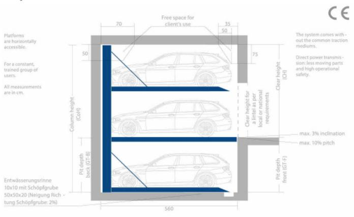
Pit length 555 cm, for 500 cm long cars. Further dimensions upon request. Concrete: min. 18, C25, floor evenness acc. to DIN 18202 Tab. 3, line 3. Load per parking space: max. 2.000 kg, wheel load: max. 500kg. Optional up to 2.300 kg or max. 2.600kg, wheel load max. 650kg.
