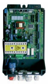
Modular extension by means of: Module 1 LC double detector Module 2 Rolling code radio remote receiver Module 3 LCR relay board
